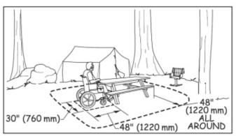
Recommend providing a 36" min. by 48" min. stable, firm and slip-resistant surface adjacent to at least one bench in each area where benches are provided positioned to allow a person in a wheeled mobility device and a person sitting on the bench to have their shoulders aligned in a manner that is substantially similar to what is shown in the following diagram.
