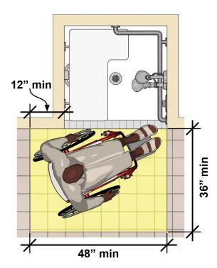
**Note:** The required clearance must be located so that it aligns with the control wall and extends 12" minimum from the seat wall. This allows proper alignment with the seat for transfer from wheelchairs.
