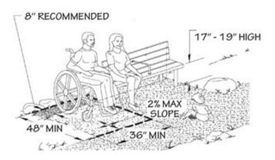
**Figure 1** shows a stable, firm and slip-resistant surface adjacent to a bench positioned to allow a person in a wheeled mobility device and a person sitting on the bench to have their shoulders aligned:
