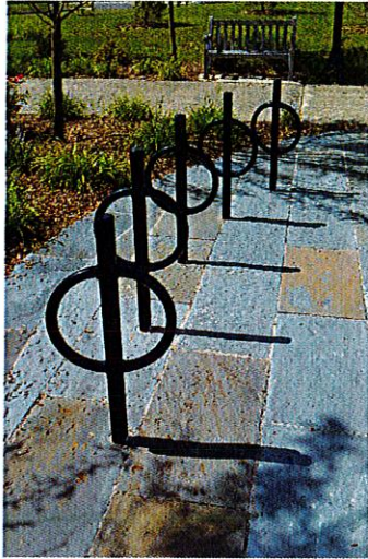
Figure 7. U-style bike racks (as seen in top image) or ring style bike racks (above) are encouraged. (Dodson & Flinker)
